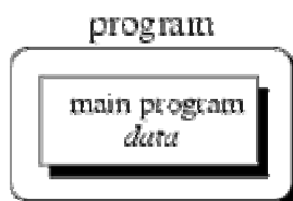
Figure 2.1: Unstructured programming. The main program directly operates on global data.
