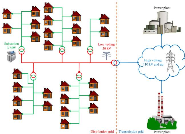
Fig. 2. Conceptual view of the framework adapted to the current structure of the electrical grid.
